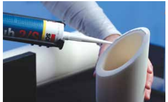
2.2 Apply sealant to the two halves and press firmly together to make the elbow fitting.
