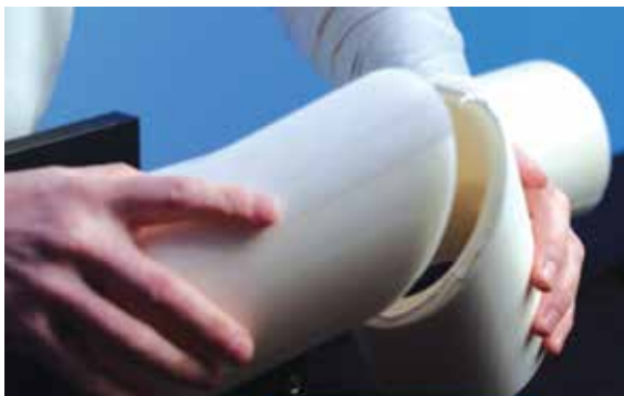
2.3 A minimum period of 6 hours is needed for the sealant to cure. All elbows and fittings must be fabricated with the use of sealant.
